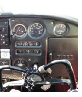
I start my takeoff roll with one notch of flaps (10 degrees) until I have flying speed. Then I put the second notch in (25 degrees) and pull back enough to get into ground effect. I climb at best angle of climb ( $V_x$ ) if I have to, but many back-country strips have departure routes that allow shallower angles of climb. Make sure you know your aircraft well and get backcountry instruction before going in there alone.
